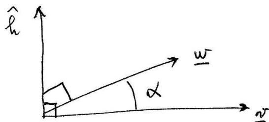
Dot product :  $\underline{v} \cdot \underline{w} = v_1 w_1 + v_2 w_2 + v_3 w_3 = vw \cos \alpha$
