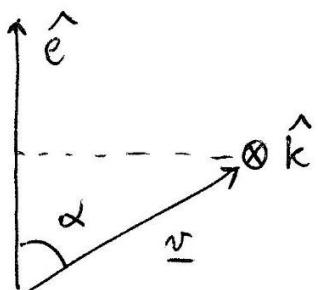
$$\frac{\Delta \underline{v}}{\Delta t} \xrightarrow{\Delta t \rightarrow 0} \frac{d \underline{v}}{dt} = v s_{\alpha} \frac{d \theta}{dt} \Big|_{\Delta t \rightarrow 0}$$
