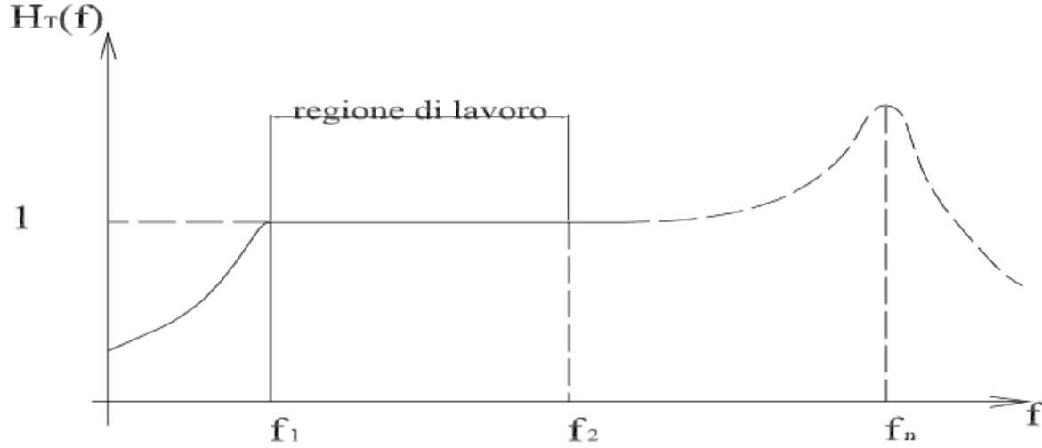
Figure 1.6: Effective bandwidth of a piezoelectric accelerometer.
