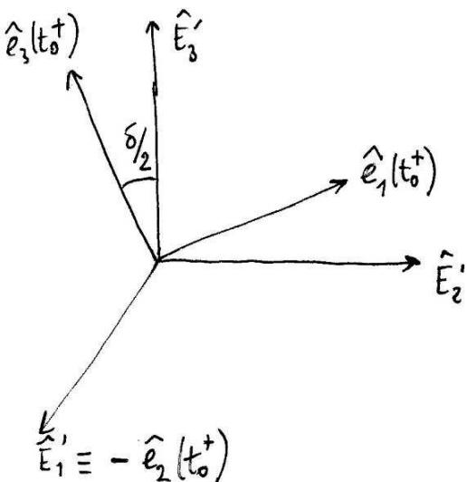
$$\left\{ \begin{array}{l} \dot{\psi} = \frac{I_3}{I_T} \frac{\omega_{30}}{G} \\ \dot{\theta} = 0 \\ \dot{\phi} = \omega_{30} \left( 1 - \frac{I_3}{I_T} \right) \end{array} \right. \quad \theta = \frac{\delta}{2}$$
