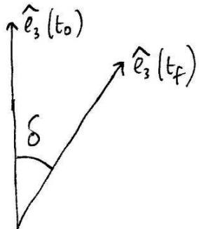
$\hat{e}_3(t_0)$  and  $\hat{e}_3(t_f)$  are displaced by  $\delta = 15 \text{ deg}$  and at  $t_f$   $\underline{\omega} = \omega_{30}\hat{e}_3(t_f)$
