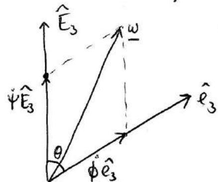
In both cases  $\hat{e}_3$  rotates in counterclockwise sense around  $\hat{E}_3$  together with  $\underline{\omega}$  that rotates as well.
