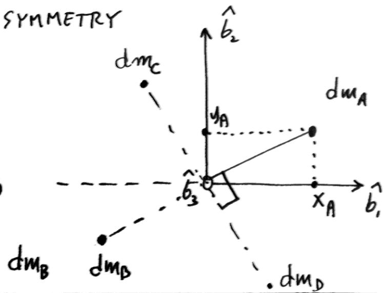
4 equal small masses  $dm_A = dm_B = dm_C = dm_D = dm$  ster
