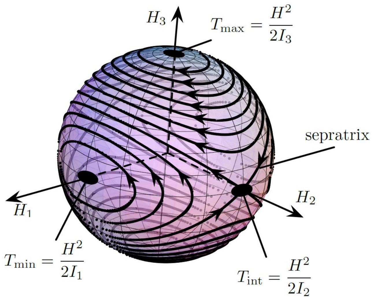
Finally, as  $T_{\text{rot}}$  approaches  $T_{\min}$ , the rotation tends to become pure spin about the maximal inertia axis, which is the only stable configuration when dissipation is considered.
