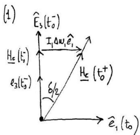
$$\underline{H}_c^{(E)}(t_0^+) = \begin{bmatrix} I_1 \Delta \omega_1 \\ 0 \\ I_3 \omega_{30} \end{bmatrix}$$
