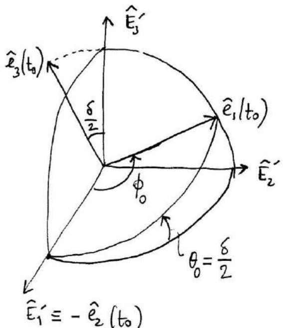
The choice of  $\hat{E}'_2$  and  $\hat{E}'_3$  is arbitrary. However, if  $\hat{E}'_1$  is chosen as aligned with  $-\hat{e}_2(t_0)$ , one can easily recognize that the values of the Euler angles at  $t_0$  are
