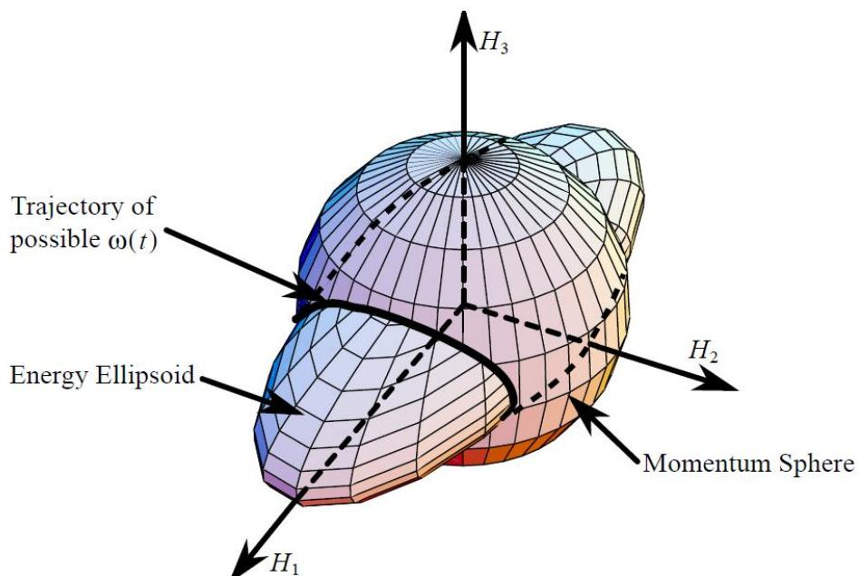
Given  $\underline{H} = \text{const}$ ,  $|\underline{H}|^2 = \text{const}$ , only a given range of angles corresponds to feasibility.
