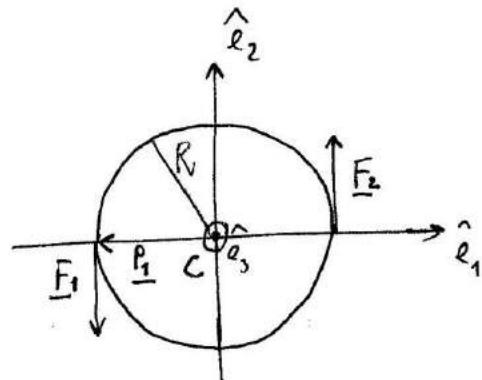
Thrusters for attitude are ignited in pairs, like in the above figure. In this way, no effect on the motion of the center of mass is produced. Conversely, the two forces  $\underline{F}_1, \underline{F}_2$  yield a torque about the mass center C
