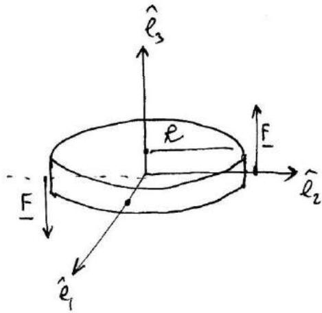
In order to provide the impulsive change  $I_1 \Delta \omega_1$ , the impulsive torque is  $2FR$
