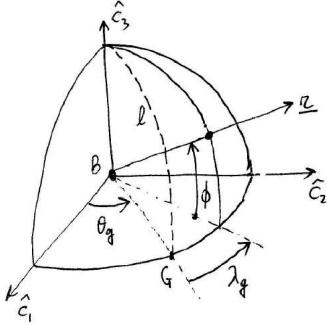
I is the Greenwich meridian identified by its abolute longitude  $\Theta_g = \Theta_{go} + \omega_E (t-t_o)$ ( $\omega_E = E$  anthe rotation rate)
