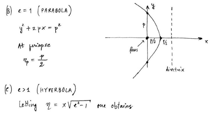
$$\begin{split} \eta^{2} - 2ep \frac{\eta}{\sqrt{e^{2}-1}} &- y^{2} = -p^{2} \quad i.e. \\ \eta^{2} - 2ep \frac{\eta}{\sqrt{e^{2}-1}} &+ \frac{e^{2}p^{2}}{e^{2}-1} &- y^{2} = -p^{2} + \frac{e^{2}p^{2}}{e^{2}-1} \\ \left[\eta - \frac{ep}{\sqrt{e^{2}-1}}\right]^{2} &- y^{2} = \frac{p^{2}}{e^{2}-1} &\longrightarrow \left[ \times \sqrt{e^{2}-1} - \frac{ep}{\sqrt{e^{2}-1}} \right]^{2} - y^{2} = \frac{p^{2}}{e^{2}-1} \end{split}$$
