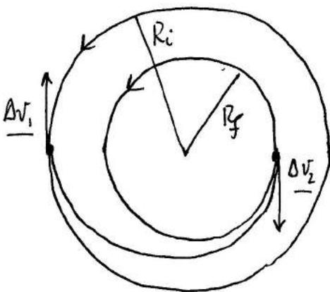
$$\Delta v_1 = \sqrt{\frac{\mu}{R_i}} - \sqrt{\frac{\mu}{a_T} \frac{1-e_T}{1+e_T}}$$
