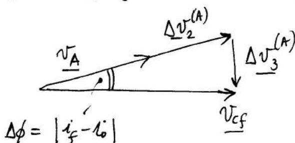
$\underline{v}_A$  = velocity at apoapse (after first impulse)
