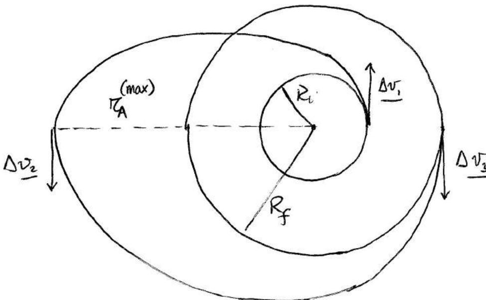
$\Delta v_1$  and  $\Delta v_2$  in the direction of motion (they yield an orbit with a greater semimajor axis)
