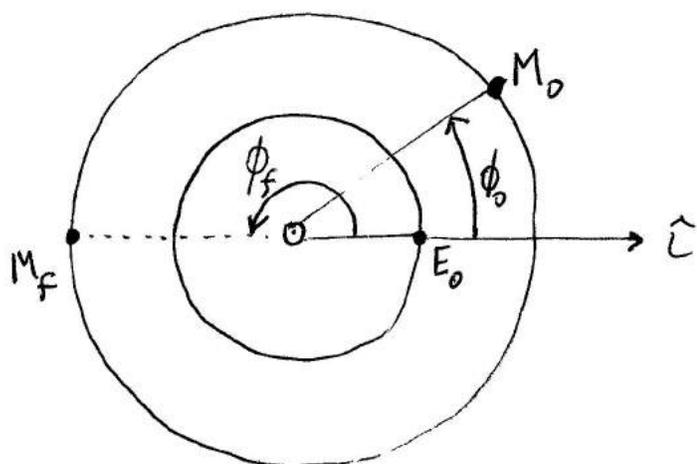
If the Earth is located as in the left figure ( $E_0$ ), which is the correct phasing (angle  $\phi_0$ ) of Mars at to such that planet encounter can occur?
