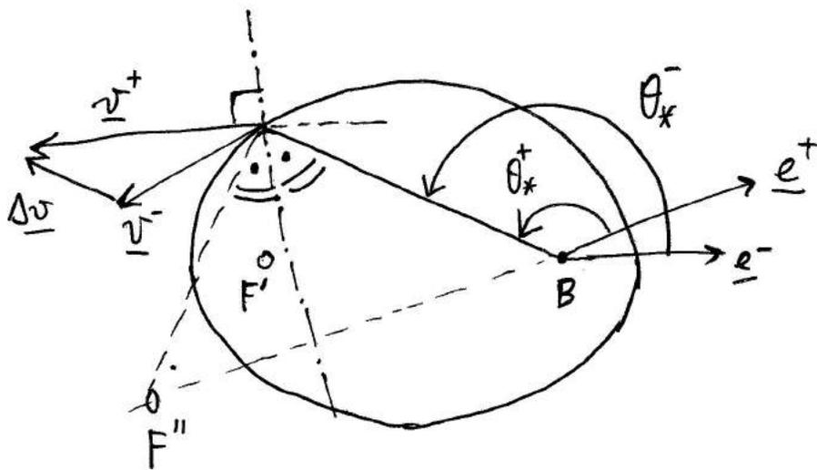
The apsidal line ( $\parallel \underline{e}$ ) is rotated by angle  $\theta_x^- - \theta_x^+$
