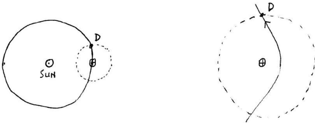
Relative to Earth the trajectory is a hyperbola. However, at the sphere of influence (where Earth attraction "ceases", i.e. becomes less important than solar gravitational attraction), point D, the spacecraft has velocity  $v_{\infty}$  relative to the Earth. If this  $v_{\infty}$  has a proper direction, the spacecraft travels in a heliocentric elliptic trajectory toward the destination planet
