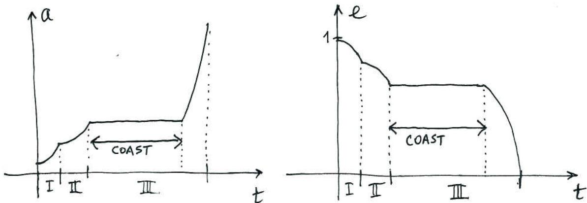
Right after launch,  $e \approx 1$ , i.e. the trajectory is nearly-rectilinear.
