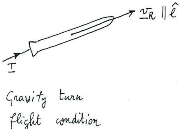
As the thrust direction is usually near-coincident with the longitudinal axis, the gravity turn condition implies aligning  $\underline{T}$  (thrust direction) and  $\underline{v}_R$  (velocity relative to the atmosphere)
