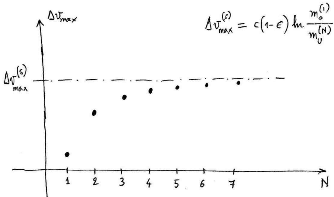
Increasing the number of stages implies increasing  $\Delta v_{\max}$
