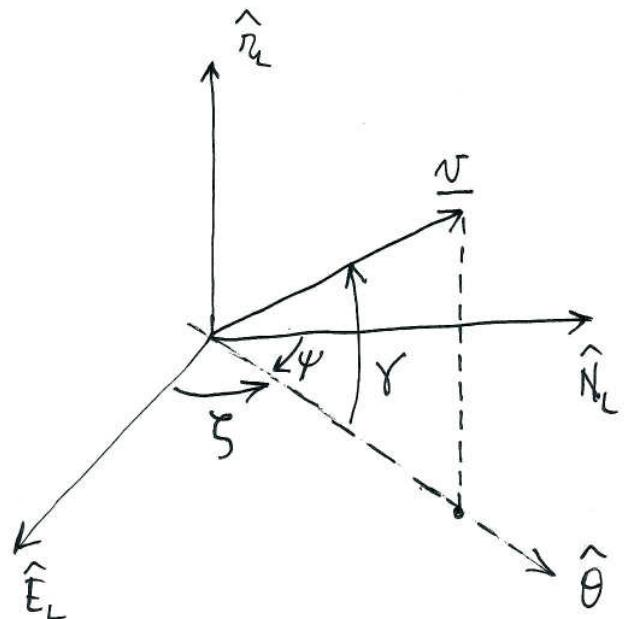
$\gamma$  = flight path angle     $\zeta$  = heading angle
