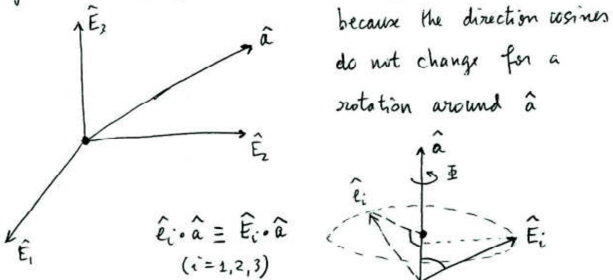
$\hat{E}_i$  rotates along the dotted line and its component on  $\hat{a}$  does not change
